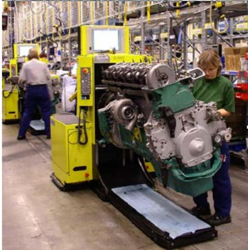
Fig. 3: The AGV/carrier and its cargo, a diesel engine.
